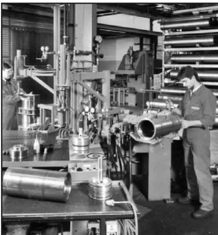
Assembly of Piston Accumulators
