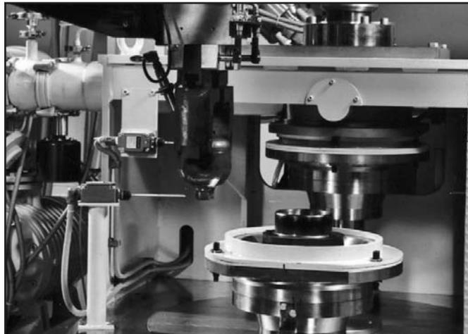
Electron-beam welding of diaphragm accumulators
