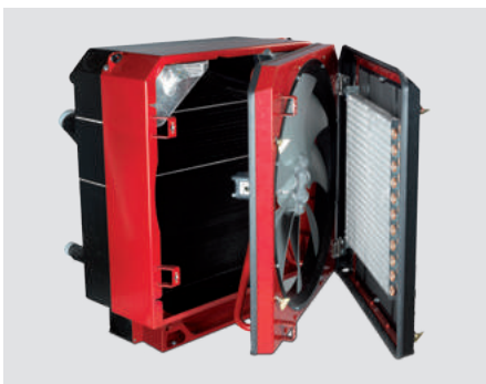
Combination cooler for forestry machine: air cooler for 4 cooling circuits with fine filter grille, in folding design for easy, tool-free cleaning
